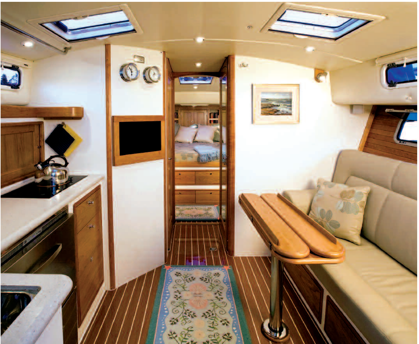
Top left: The portside navigation console is equipped with an optional wide Stidd chair facing a large chart flat and VHF radio. Top right: The helm features a Raymarine C120 wide-screen MFD, electronic engine controls, and a joystick for the IPS drives. Above: The well-ventilated main saloon has a full galley to port and a settee to starboard that converts to Pullman-style berths.
