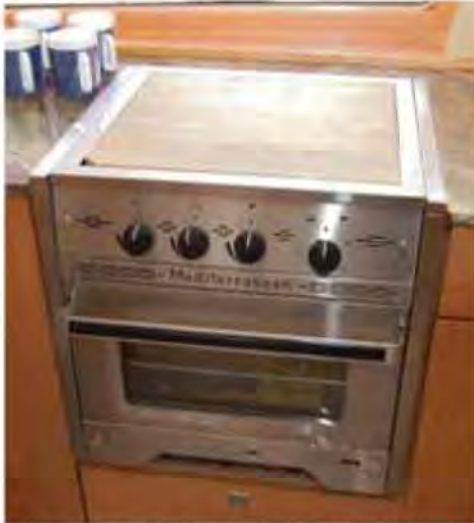
A propane stove and oven eliminates much of the need to run a genset at anchor.
