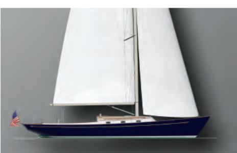
He says he tried to keep the design simple. The weather deck layout is clean, save for the raised cabin top. Zurn says the intention was to make it easy for a single person to handle the boat, and let the passengers be passengers.
